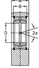
$\begin{array}{lll} A & = 180 \\ a \text{ (degrees)} & = 6 \\ B & = 55 \\ D & = 80 \\ Dynamic load C \text{ (kN)} = 400 \\ F & = 141 \\ L & = 231 \\ M & = 60 \\ \end{array}$
